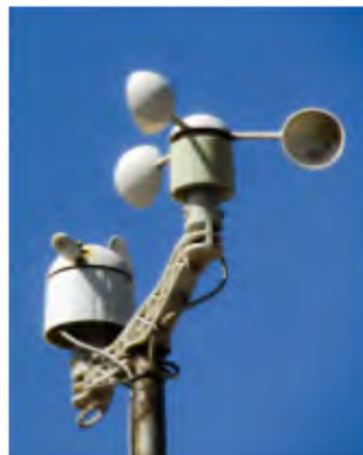
Anemometer Measures wind speed
