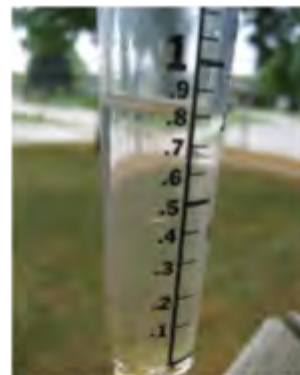
Rain Gauge Measures amount of precipitation
